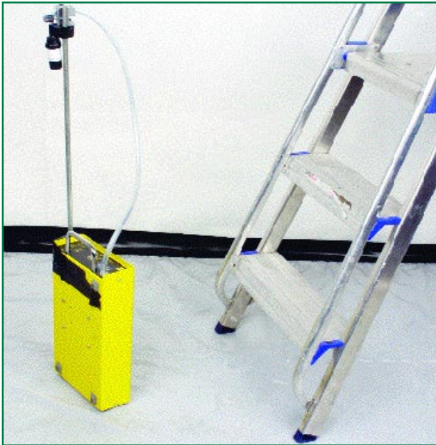
Figure 6.6 Air sampling during clearance
