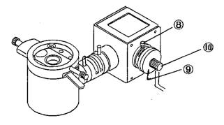
To move the bulb horizontally, turn the Lamp Centering Control (10)
